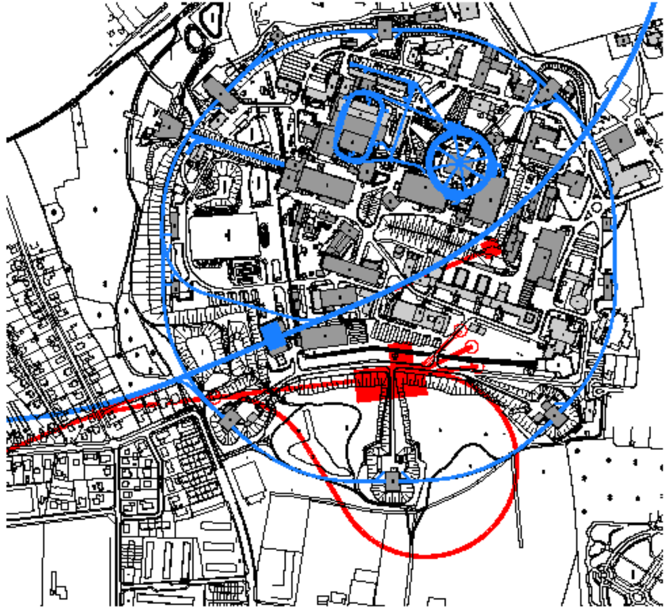
Figure 2.3.2: Site of THERA: TESLA (red) is foreseen to be built tangentially to the HERA ring (blue) such that electrons from North hit protons in the West Hall on the DESY site. The PETRA ring is seen which serves as a pre-accelerator for HERA protons. The PETRA lepton injection line will be instrumented with superconducting magnets to arrange protons travelling clockwise in HERA. After collision the TESLA electrons will be dumped on site.
